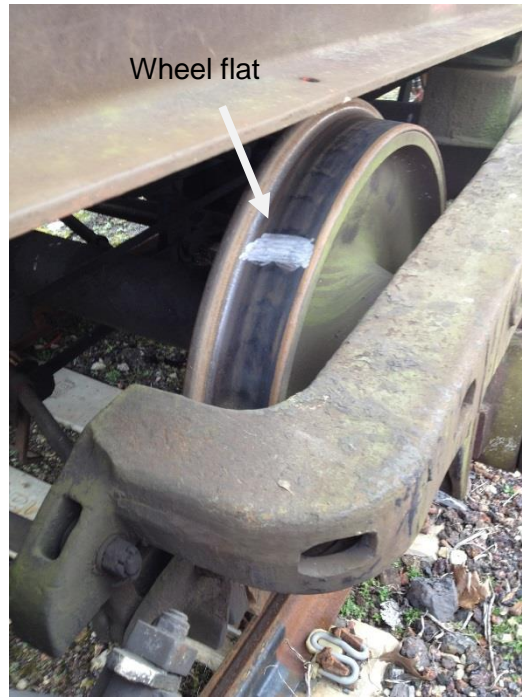
Figure 7-3: Artificially induced wheel flat in the field experiments.
