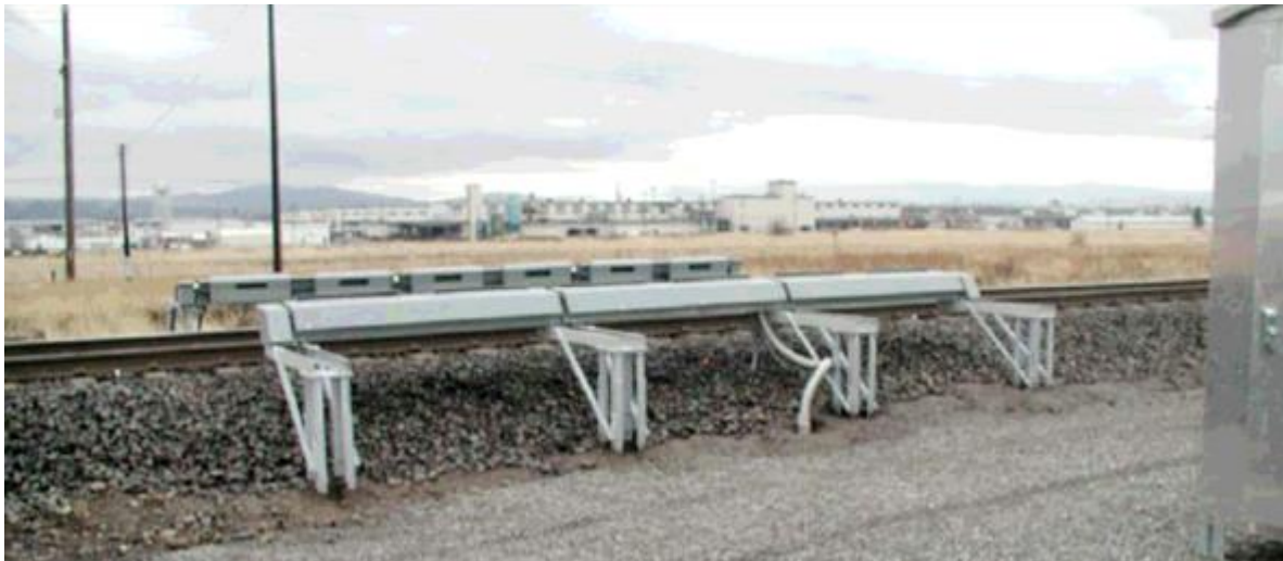
Figure 3-3 : The trackside acoustic detector system [48].
