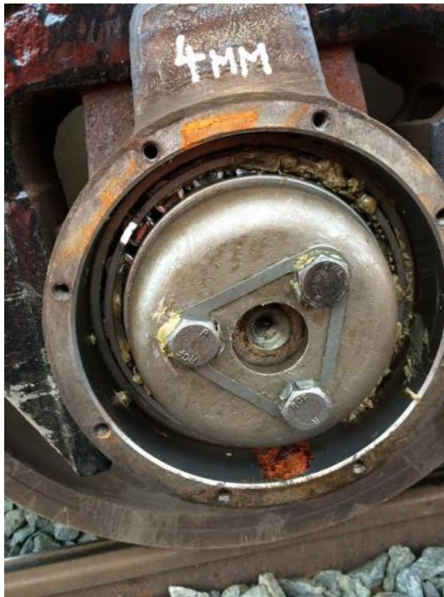
Figure 6-2: Example of a defective bearing with 4mm roller defect
