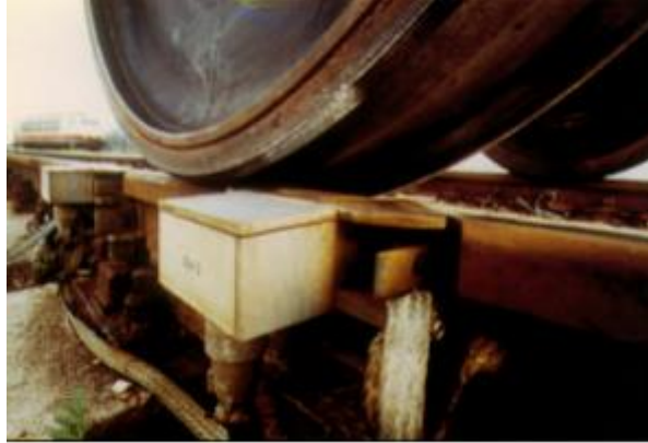
Figure 2-14: EMAT-based system installed on-track for the online inspection of the rolling surface of the wheels [1].
