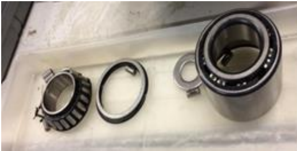
Figure 5-26: Example of a rig double-row tapered roller bearing.
