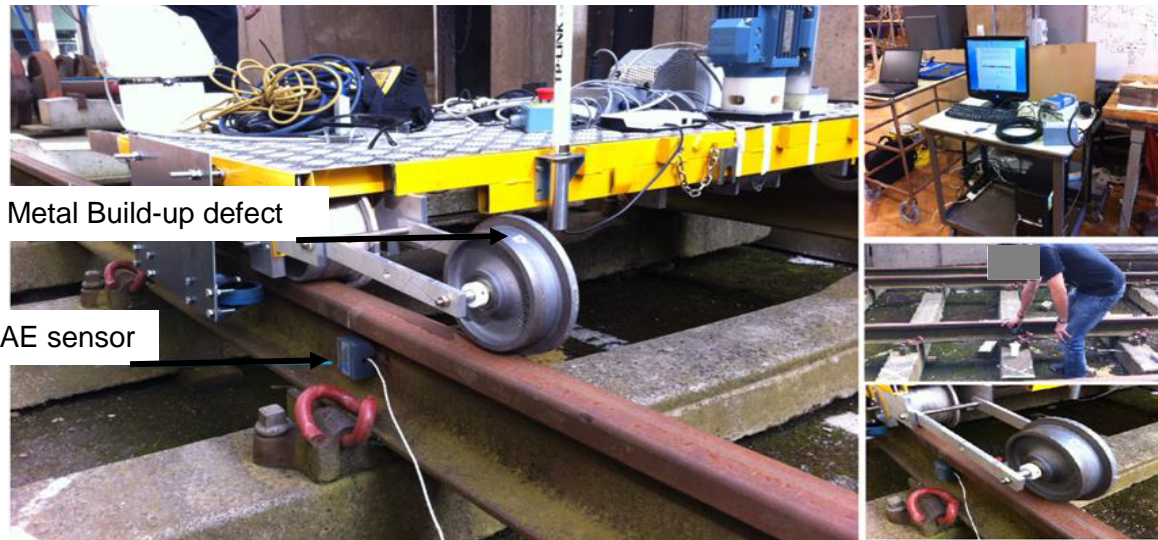
Figure 5-21: Experimental work with motorised trolley.
