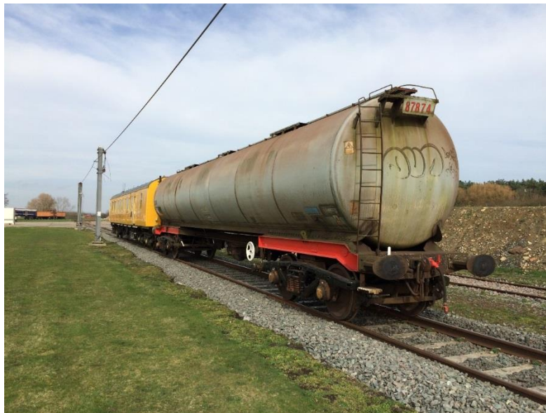
Figure 6-11: Test car in Long Marston test field. The yellow locomotive in front pulls or pushes the test wagon depending on the direction of movement.
