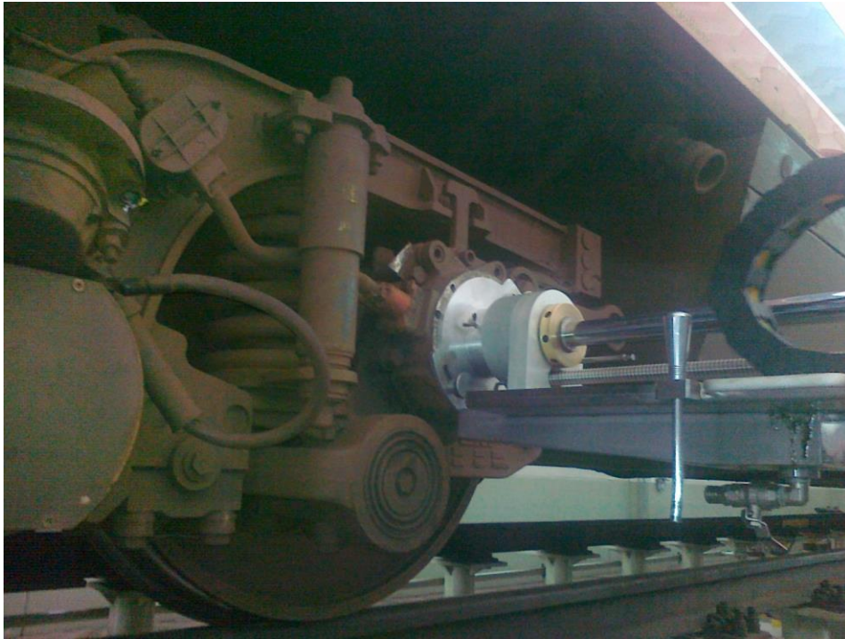
Figure 2-11: Ultrasonic inspection of a rolling stock hollow axle.
