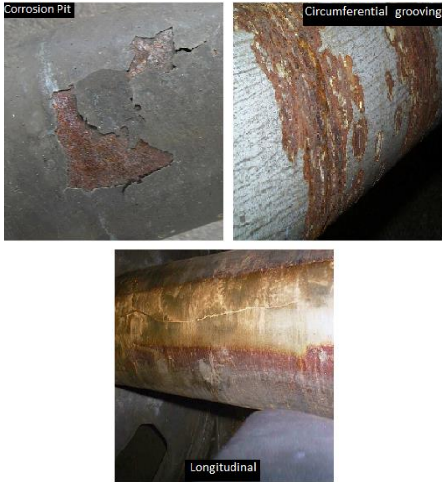
Figure 2-9: Axle defects [8].
