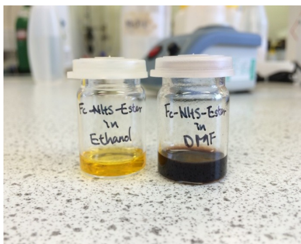
Figure 5.5.2.2.5.5 Image of FcA-Ester diluted in Ethanol (left) and DMF (right) after 2 hours.
