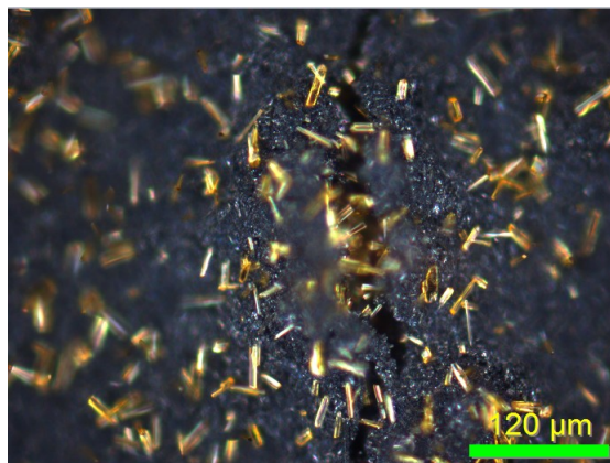
Figure 5.5.1.1.4 20 X microscopy image of 10 % w/w FcA in carbon paste hand print electrode.
