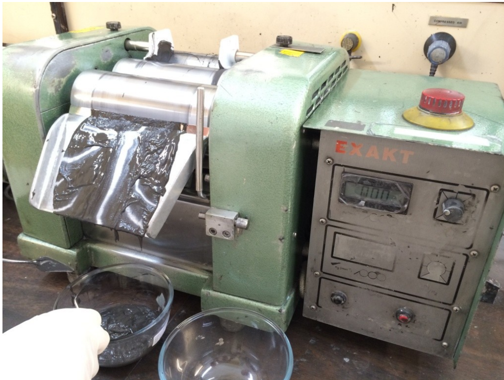
Figure 5.5.1.3.3 Example of the mixer that is used for blending mediators or enzymes into screen printing ink.
