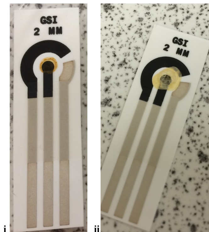
Figure 5.5.1.4.1 Image of electrode after (i) 10 mM of FcA in ethanol is dropped and dried on the working electrode and (ii) different concentration of CA membrane in 90% acetone dropped on top of the dried FcA.
