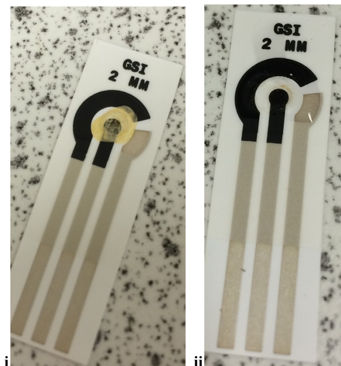
Figure 5.5.1.4.5 Image taken of 10mM FcA and CA membrane drop coated electrode (i) before and (ii) after 25 cycles of CV in PBS.
