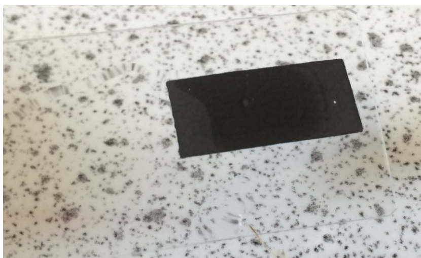
Figure 5.5.1.2.4 Image of PBS solution soaking through the screen printed electrode.
