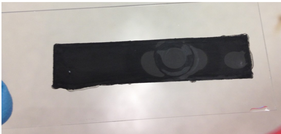
Figure 5.5.1.1.3 Photo image of the bottom of the hand screen printed electrode showing PBS solution soaking through the electrode paste.
