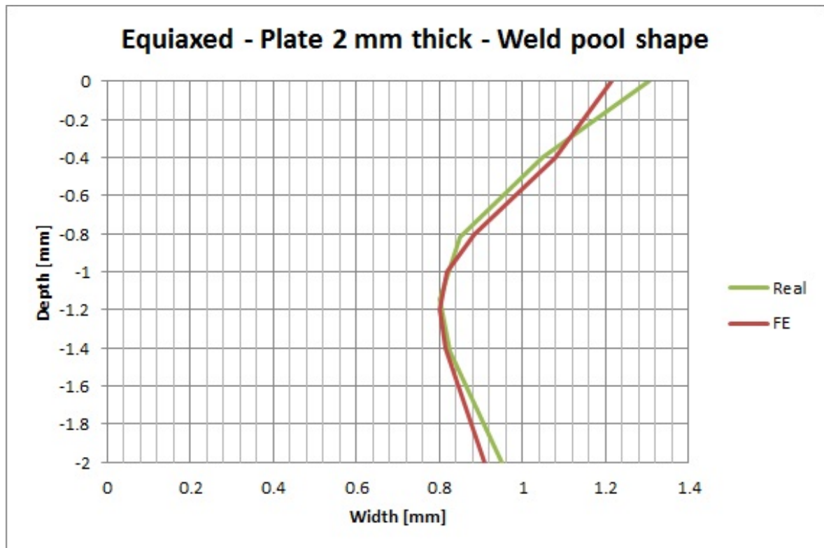
Figure 4.36.: Comparison of the weld pool shape between numerical and experiment results of the Ti-6Al-4V plate 2 mm thick with initial equiaxed microstructure (figure 4.35). Only one half is shown as the shape of the weld pool is assumed to be symmetric
