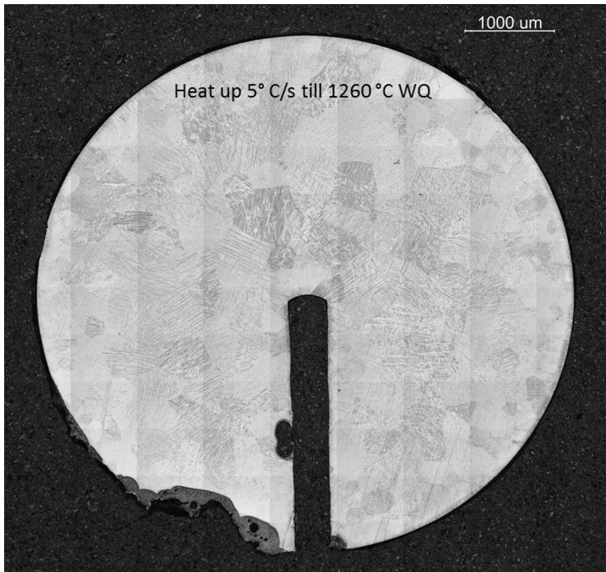
Figure B.1.: Montage of the sections taken at the optical microscope for the sample tested at a heating rate of 5 °C/s till 1260 °C then water quenched. The irregular surface close to the vertical hole is due to the spot welding of thermocouples in that area
