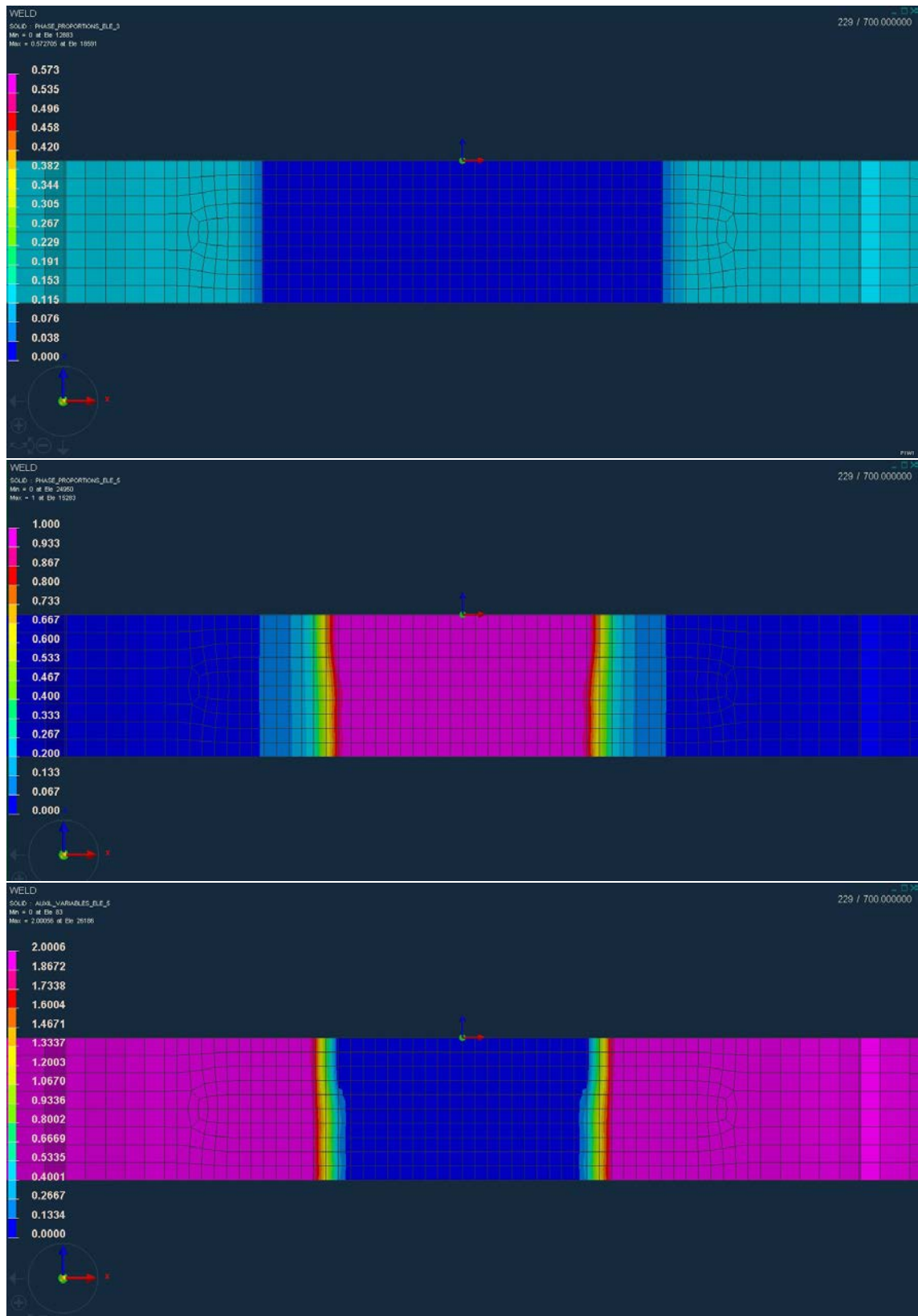
Figure 5.2.: \beta phase proportion (top), martensitic phase proportion (centre) and radius [ \mu\text{m} ] of the \alpha equiaxed microstructure (bottom) obtained running the FE welding simulation with conditions described in figure 5.1 (plate 1 in table 5.1)
