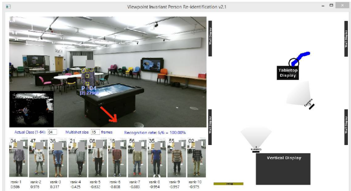
Figure 6.3. A person arrives at the tabletop display. ViMM identifies this person as having an ID=04. Location tracking is marked on the map by the blue trail.
