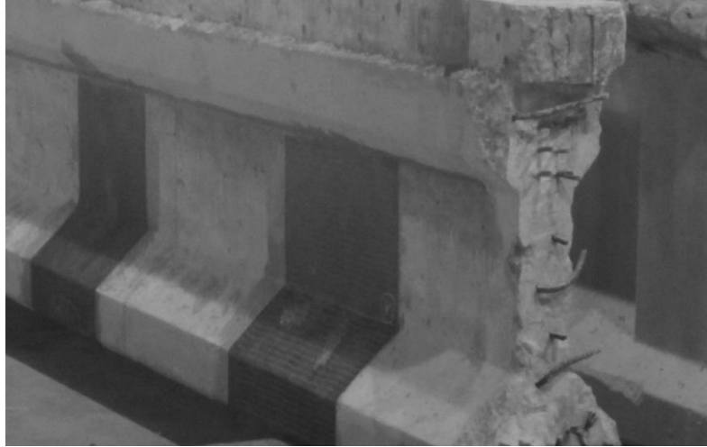
Figure 3.11 – Example of different U-wrap widths for girder 6
