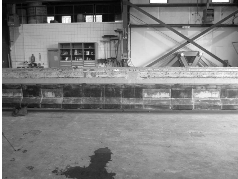
Figure 3.10 – Finished repair of test girder in the lab
