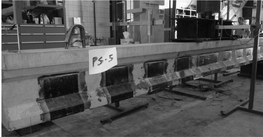
Figure 3-19: Testing Setup Photo for Statically Loaded PSC Girders
