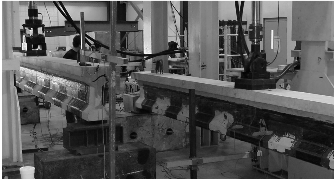
Figure 3-21: Testing Setup Schematic for Dynamically Loaded PSC Girders
