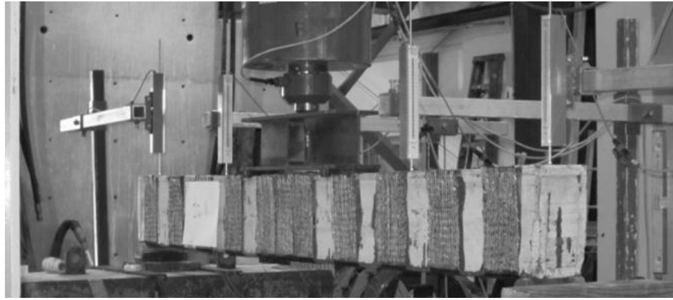
Figure 3-16: Example of Testing Setup for RC beams
