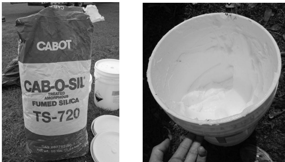
Figure 3-14: (left) Fumed Silica used to Thicken Epoxy; (right) Thickened Epoxy
