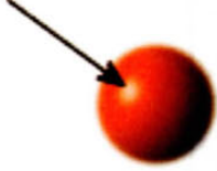
Figure 5. Specular color on a sphere, the shiny exponent will effect the area of the Specular “spot”.
