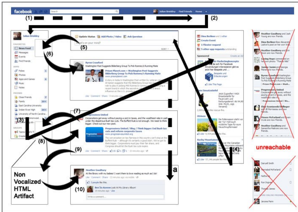
Figure 7: Exploded view of the standard UI demonstrating the order in which content sections are vocalized by the ChromeVox screen reader (numbered 1 – 10).
