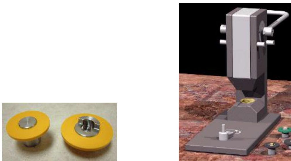
Figure 7.1: T zero sample press and pans used to seal samples for DSC experiments.
