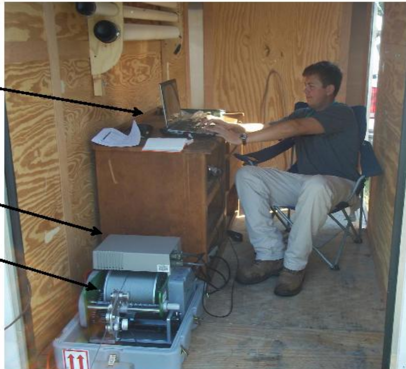
Figure 22. Interior of ECU geophysical logging trailer with tools and instruments employed during well logging. Alex Culpepper pictured operating winch using MATRIX software.
