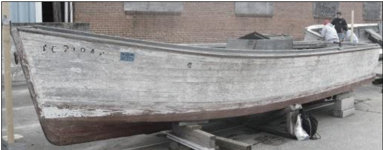
Figure 26. Deadrise, V-bottom, or “round chine” shad boat now located at Plymouth, NC. (Photo by Dan Brown, 2010).
