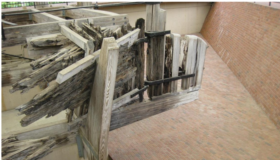
Figure 17: U.S.S. Cairo at Vicksburg, port side rudder (photo taken by Melissa Ashmore) 3
