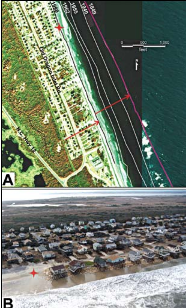
FIGURE 11. Panel A is a 1998 aerial photograph of a portion of South Nags Head on Bodie Island and displays the location of the 1849 shoreline (red line) relative to the shoreline location in 1998 (black line). The location of the shoreline is shown in a recessional sequence for 1940, 1955, and 1962 (white lines). Panel B is an oblique aerial photograph (2008) that shows a housing development built in the 1980s, encased in sand-bags for several decades, and the receding shoreline adjacent to the houses. The red star is the same location on both panels. Panel B photograph is by S. Riggs.
