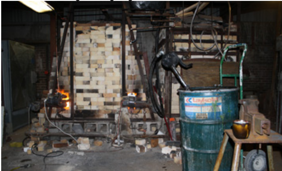
Photo 6 – Cat firing with zig-zag lines to burners
