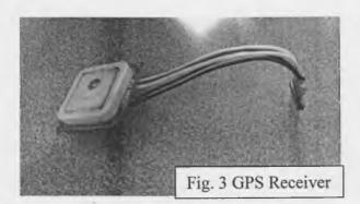
For the Smart Cane's audible GPS system it was implemented to allow the user to accurately pin point where they are on campus. Also, the design will output an audible response when in range of buildings on campus. For this design a 66 Channel LS20031 GPS 5Hz Receiver was used. The LS20031 includes an imbedded antenna and GPS receiver circuits. It can output positional information every second. In our design it is used at its this limit. This GPS can track up to 66 different satellites.
