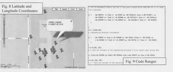
After finding the latitude and longitude ranges around the Engineering building and two subsequent smaller ranges around each of the Engineering building's two main entrances the audible code was constructed. The code was to make the piezo to vibrate at different frequencies to make different
