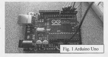
The Arduino was coded was to emit a burst of ultrasonic noise (40kHz). The ultrasonic transmitter and receiver is a HC-SR04 Ultrasonic Ranging Module. This model was easily integrated with the Arduino and the code that was written for the ranging module. The
