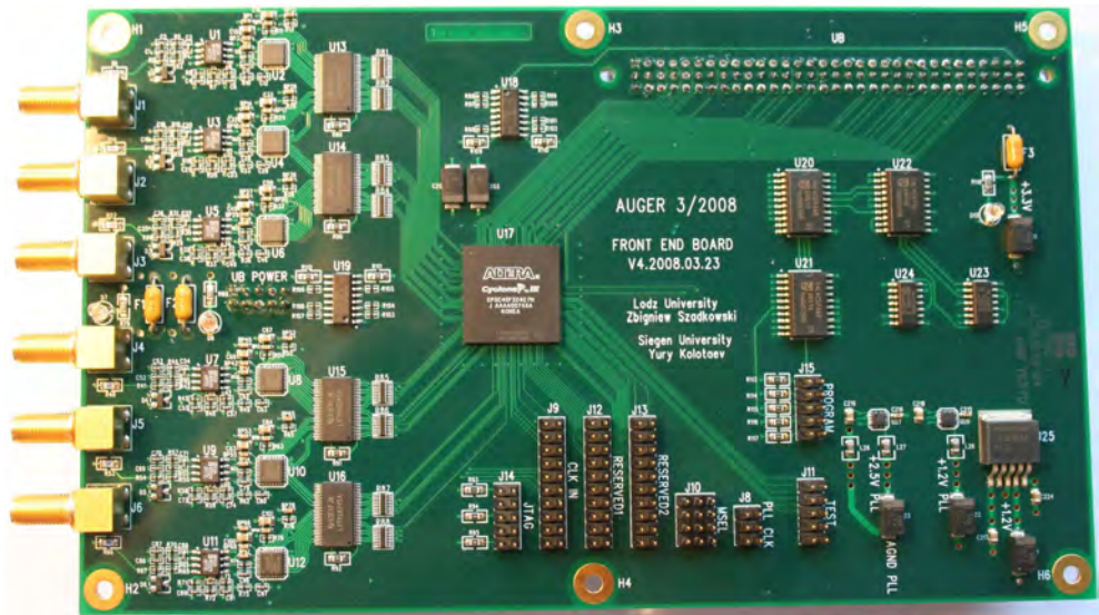
Figure 11. The 4 th generation of the Front-End Board with CycloneIII® FPGA EP3C40F3247. The EP3C40F3247 contains DSP blocks and it is possible to implement even a sophisticated algorithm like DCT engines for a recognition of horizontal or very inclined showers. This board has been used also for preliminary testing of the wavelet trigger and the signal filtering based on a chain: FFT+Median filter+iFFT.
