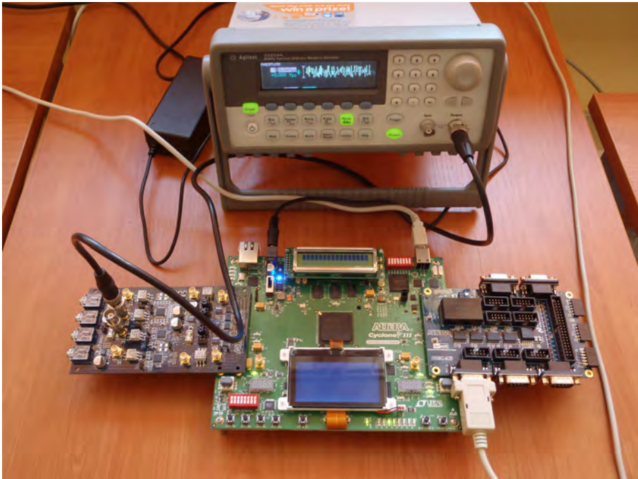
Figure 13. The test system based on a development kit with Altera® CycloneIII® FPGA EP3C120F780C7 supported by two daughter boards: AD/DA Data Conversion Card (left) with two ADCs (150MHz sampling) and two DACs (250 MHz), as well as the Industrial Communication Board (ICB-HSMC)(right) allowing a connection via the galvanic isolated RS485 ports.
