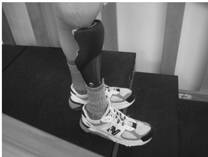
Figure 5. The initial position is to place the midfoot of the prosthetic foot at the leading edge of the step.
