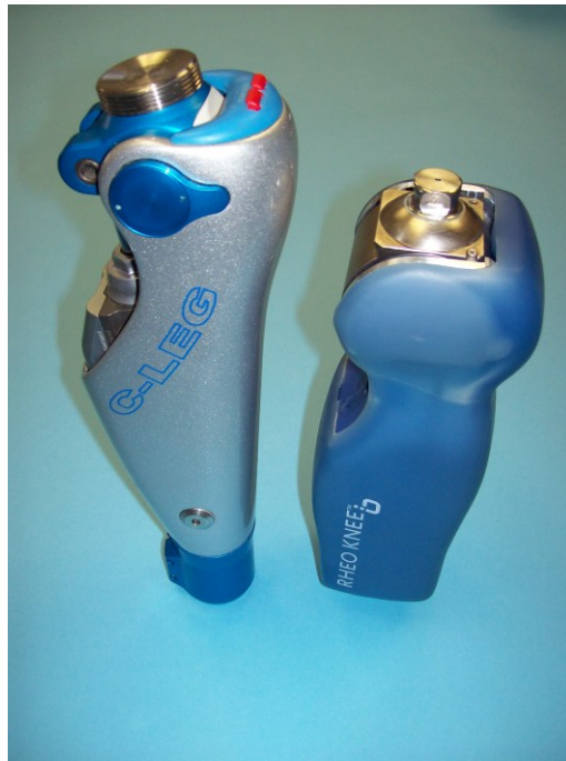
Figure 2.2. Otto Bock 3C88 C-Leg (left) and Ossur Rheo Knee). They are examples of highly technical, modular, microprocessor controlled knee units that are of a single axis design.
