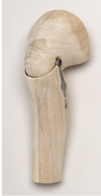
Figure 2.3. Otto Bock exoskeletal Single Axis 3P19 knee. The knee mechanism is integrated into wooden shin and distal thigh sections. The knee mechanism is a single axis, constant friction unit. Photo courtesy of Otto Bock Healthcare.
