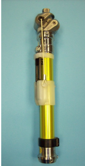
Figure 2.7. Otto Bock 3R49 knee unit. It is a single axis design with sliding, constant friction that offers only single speed cadence per setting. Stance control afforded by this unit is via weight activated stance braking. This means that after a threshold quantity of load is applied to the knee (presuming the knee is in approximately \leq 15^\circ of flexion), it will not flex further which could cause buckling. This form of stance control requires the prosthesis to be unloaded prior to swinging the leg forward. This swing requisite is commonly associated with gait deviations such as hip hiking and lateral trunk bending.
