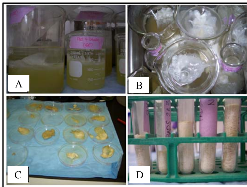
Figure 8. Images of extraction precipitation, drying and resulting mucilage. Image A and B shows the mucilage being drawn out of solution as the water is evaporated using ethanol and acetone. Image C shows the washed mucilage spread on Petri dishes to dry and D shows the final product of the extraction.
