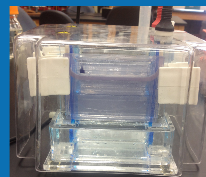
Figure 4: SDS and native PAGE gels were run using hatching liquid in this apparatus.
