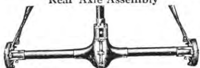
2500—Rear Axle Assembly, including drive shaft and tubing, rear radius rods, brake rods and universal joint. . . . . *78.6C
