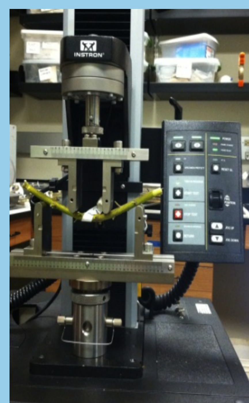
Measuring Stem Mechanical Strength using the Instron machine
