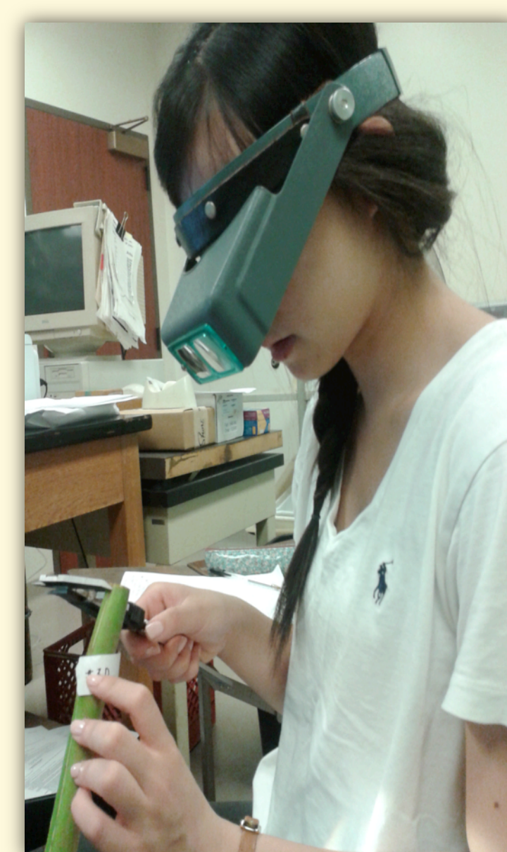
Figure 3: Careful measurements of the characteristics of each sample were taken with a vernier caliper and recorded into the Instron computer program.
