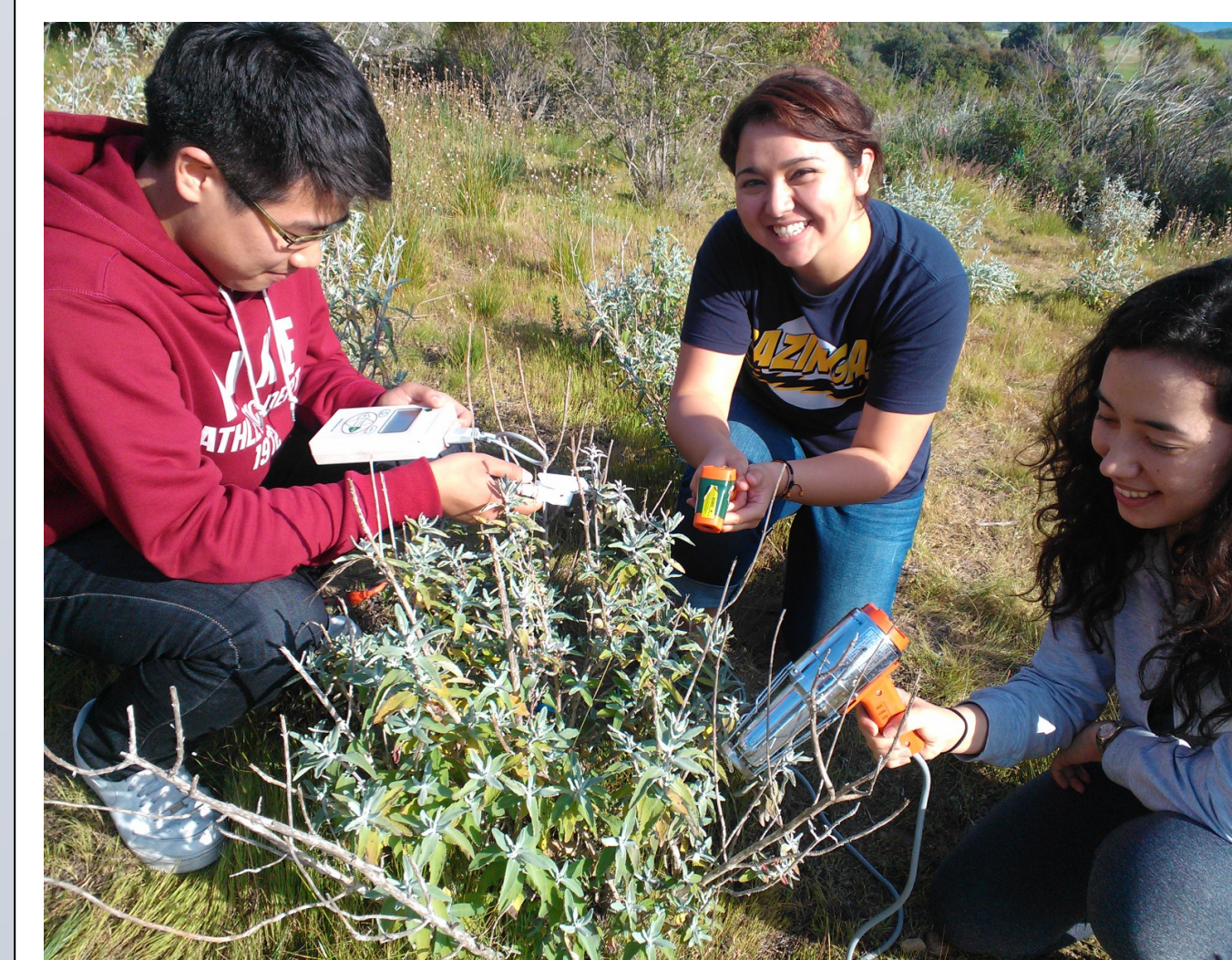
Image 5: Our group demonstrating the equipment used: porometer, IR thermometer, and heat gun.
