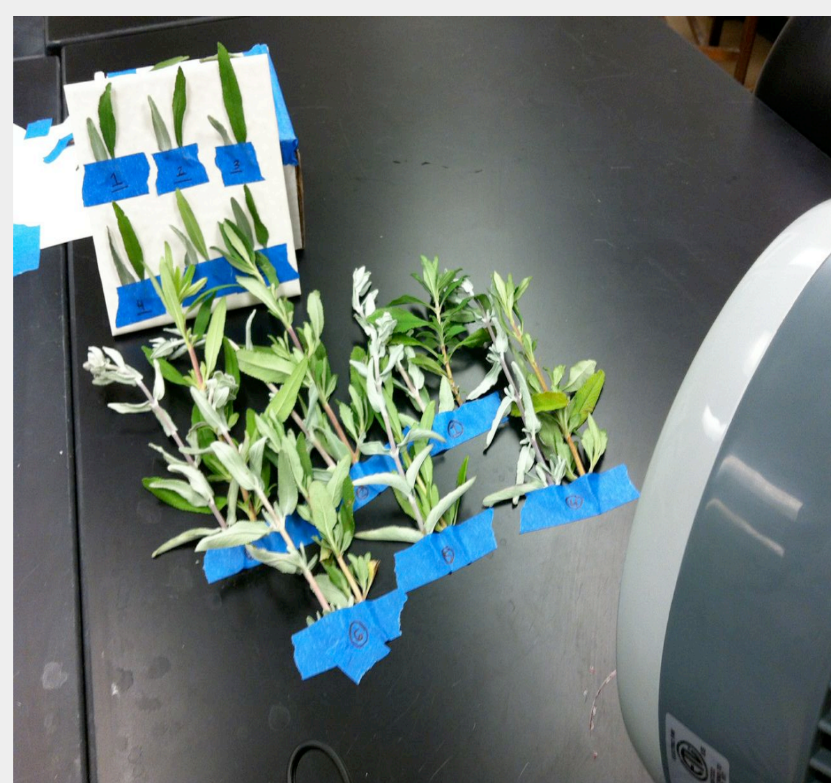
Fig.5 Experimental set up for drying. Plant type/species paired in location so that air flow was consistent through all six trials.
