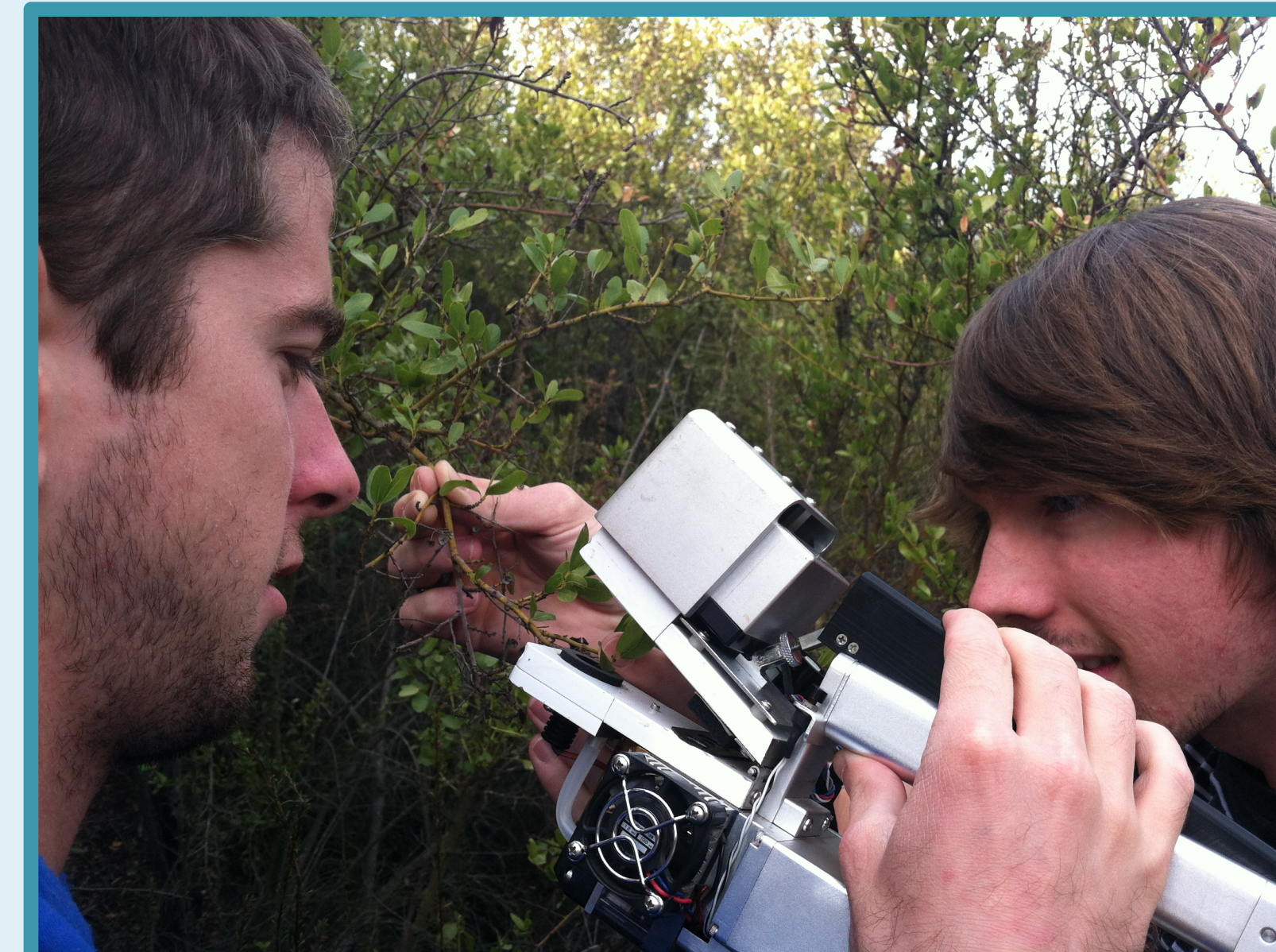
Fig. 1. To determine the photosynthesis rate of each species the LI-COR 6400 machine was used. The flow rate was set to 100 \mu\text{mol m}^{-2} \text{s}^{-1} , the CO 2 levels to 400ppm, and the temperature in the cuvette to the ambient temperature. Measurements were taken between the hours of 10 am and 12 pm
