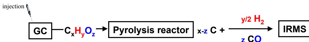
Fig. 12: Principle of compound-specific \delta\text{D} - and \delta^{18}\text{O} -analysis of biomarkers using GC-Py-IRMS. Biomarkers eluting successively from the GC-column are converted “online” in a pyrolysis reactor to hydrogen ( \text{H}_2 ) and carbon monoxide ( \text{CO} ) and the isotopic composition of these gases are determined directly in a coupled IRMS.
