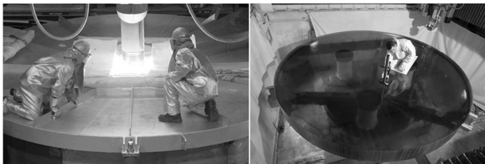
Figure 3. Casting process (left) and intermediate inspection (right) of a four-meter class ZERODUR blank
