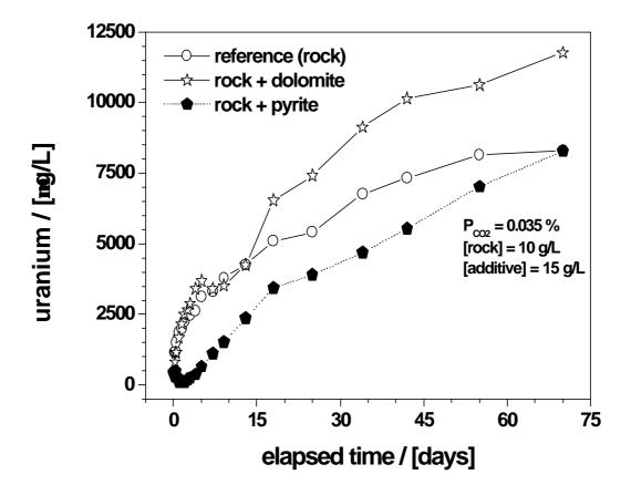
**Figure 2:** Impact of dolomite and pyrite on the evolution of uranium concentration as function of time in an air homogenized batch experiments for 70 days. Uranium is leached from a natural rock as described in ref. 36.  $P_{CO2}$  is the atmospheric partial pressure of CO<sub>2</sub> (open system). The particle size of used materials was:  $0.315 \le d$ (mm)  $\le 0.63$ . The represented lines are not fitting functions, they just joint the points to facilitate visualization.
