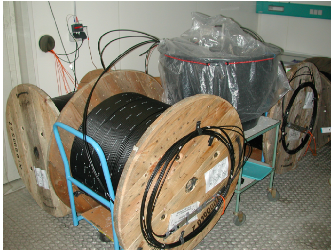
Figure A.1.: Calibration of DTS system in a temperature controlled chamber at GFZ Potsdam. 20 m of sensor cable from the cable reels are placed in a 100-liter water bath. The temperature of the water bath is measured with a precision platinum resistance thermometer. This calibration procedure results in a high stability of the temperature inside the water bath and allows for long cable sections up to about 100 m inside the bath. Nevertheless a long equilibration period is required until a stable temperature is reached, and the temperature range is limited to -15\text{ }^{\circ}\text{C} and 40\text{ }^{\circ}\text{C} . Up to two calibration measurements with different temperatures can be performed in 24 hours.
