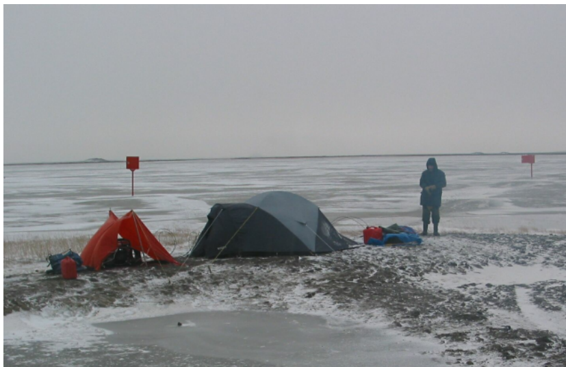
Figure A.6.: Temporary set-up of the DTS-logging equipment at the flooded and partially frozen Mallik site, Oct. 7, 2002. Foreground: shelter for DTS instrument, background: steel boxes accommodating surface ends of sensor cables (modified from Hennings et al., 2003).
