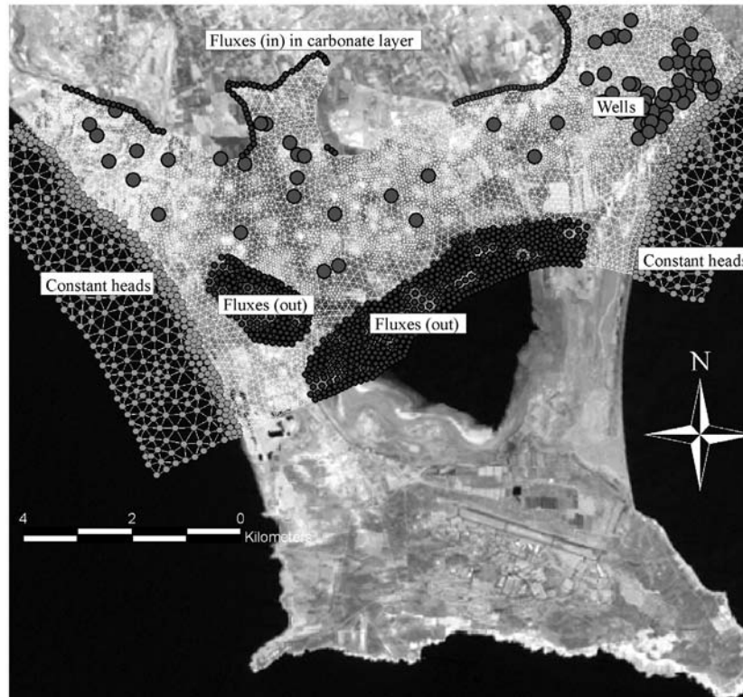
Fig. 6.8: 2-D finite element mesh and projected boundary conditions.
