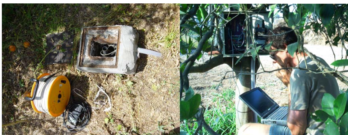
Fig. A 3.1: Monitoring well Phasouri, showing the cemented borehole head (left), and the instrument box (right) with the data logger and power supply in a waterproof box, attached to the closest orange tree.
