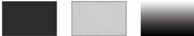
FIGURE 2.1: To illustrate the concepts of homogeneity and isotropy. In the left box, the material distribution is homogeneous and isotropic. The middle box shows a homogeneous – at large scales – but anisotropic distribution. Finally, matter in the right box is anisotropically and inhomogeneously distributed.
