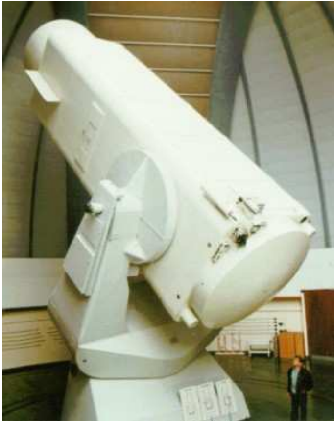
Figure 7: The 2m-Schmidt telescope of the Thüringer Landessternwarte Tautenburg, within its dome. All the optical data used within this work was taken with this telescope. (Picture courtesy of KSO Tautenburg)
