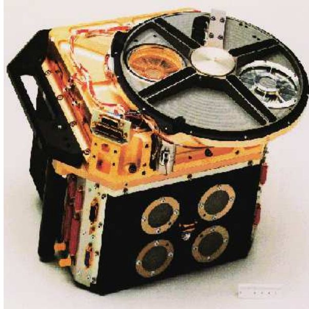
Figure 3: The ROSAT PSPC (position sensitive proportional counter) assembly, with the entrance window and filter wheel at the top. (Picture courtesy of MPE)
