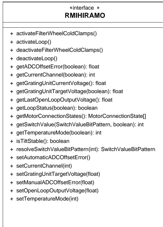
Figure 2.7: HIRAMO service interface class diagram.
