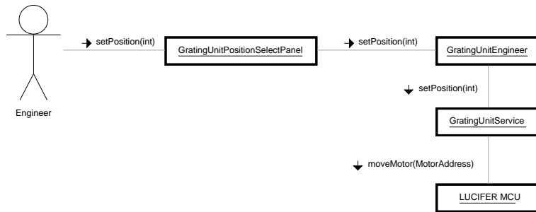
Figure 2.33: This collaboration diagram shows the involved classes when an engineer selects a new position for the GratingUnit service. The call is forwarded directly to the service by the client.
