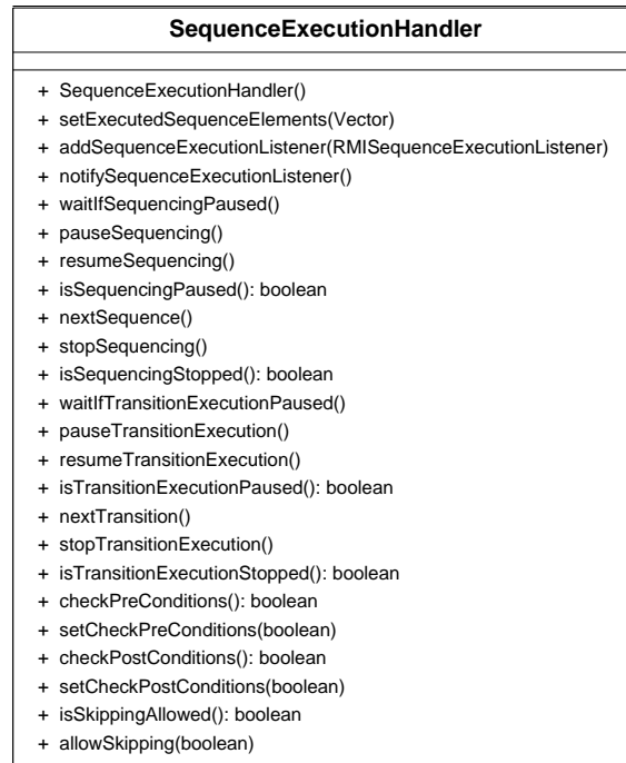
Figure 2.15: Class diagram of the SequenceExecutionHandler class.
