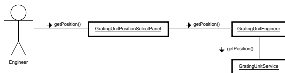
Figure 2.35: This collaboration diagram shows the involved classes when an engineer queries the position for the GratingUnit service. The call is forwarded directly to the service by the client.
