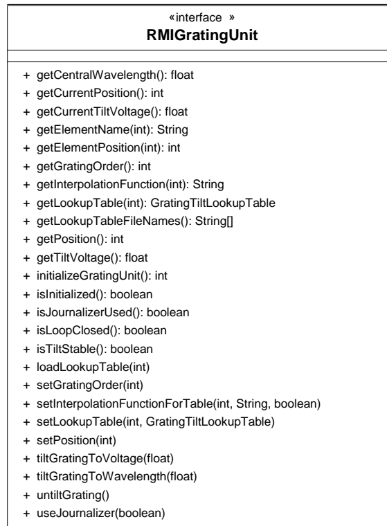
Figure 2.20: Class diagram of the GratingUnit service.
