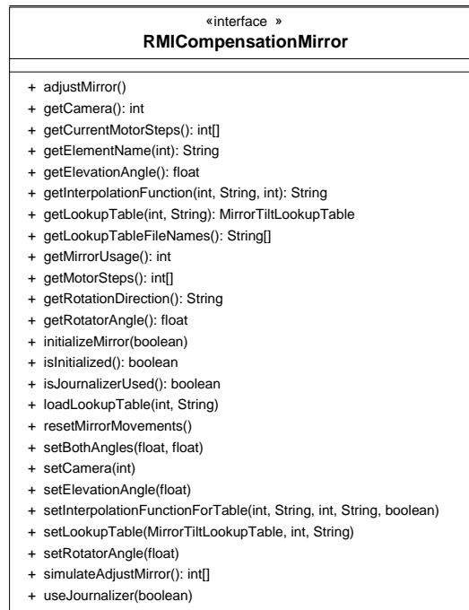
Figure 2.29: Class diagram of the CompensationMirror service.
