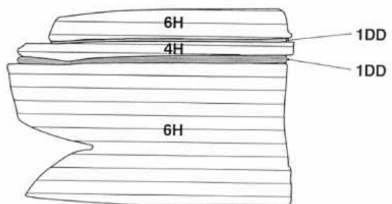
Figure 6. Illustration of the "missing piece" method of assignment for a complex sandwich SiC crystal J13.
