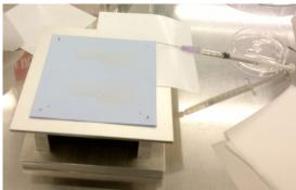
Figure 20. Aligning of the green sheets before laminating, ethanol was injected with syringe to glue green sheets together.
