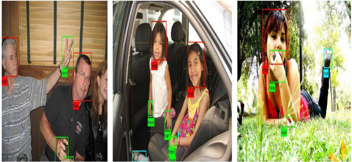
Figure 3f: Person layout challenge. Participants are expected to predict the presence of head, hands and feet in the input image.
