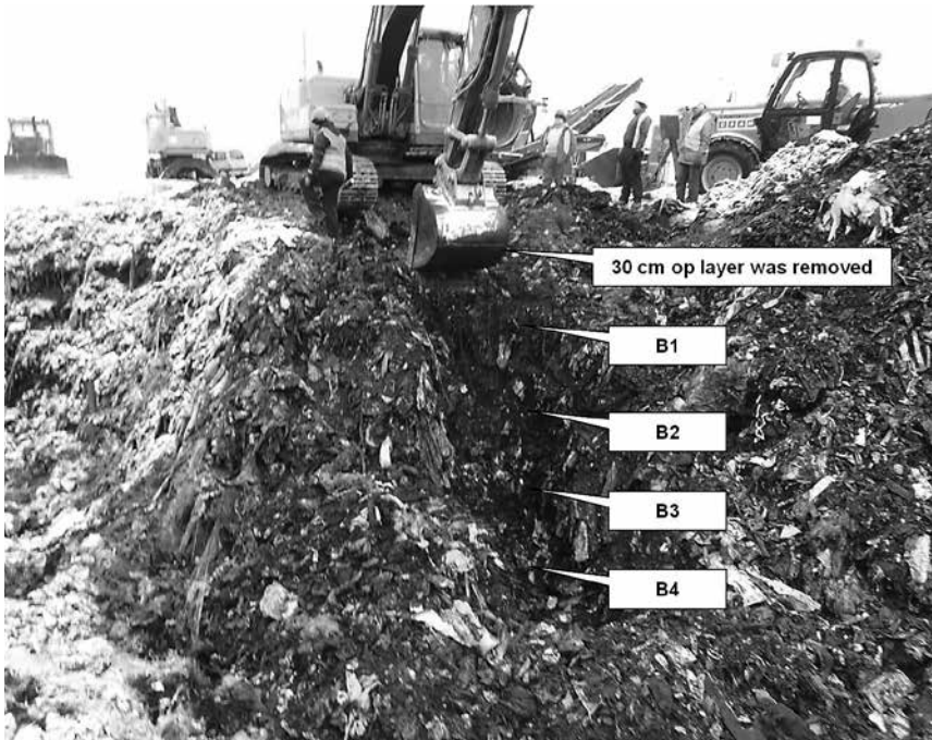
Figure 2.6. Sampling site H1 at Kudjape landfill with layers B1 to B4 as indicated
