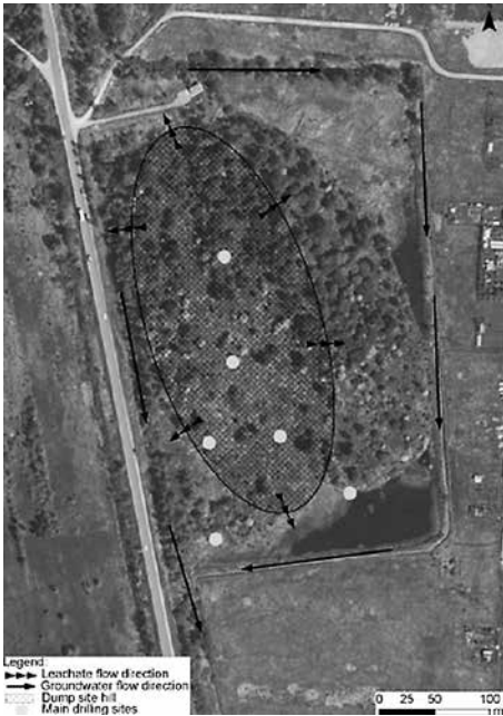
Figure 2.3. Kleisti dump site: location of drilling points; arrows indicate leachate and groundwater flow direction (as the base maps – Latvia Geospatial Information Agency ortophoto maps)
