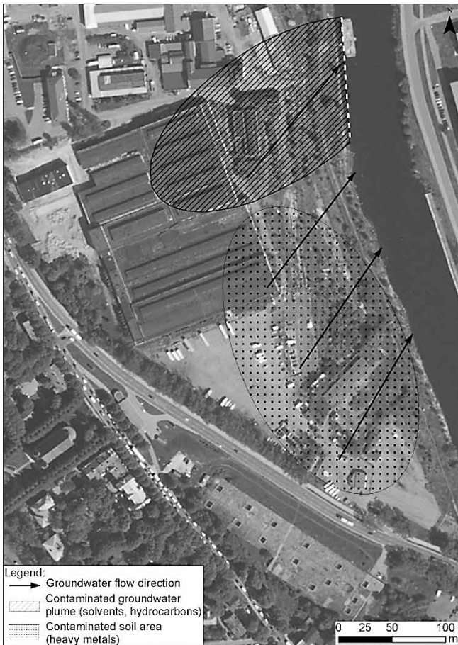
Figure 2.2. Former agricultural machinery factory “Selmash”: areas contaminated with heavy metals and solvents (two cycles of remediation were carried out in 2002-2004 and 2009); arrows indicate groundwater flow direction (as the base maps – Latvia Geospatial Information Agency orthophoto maps)
