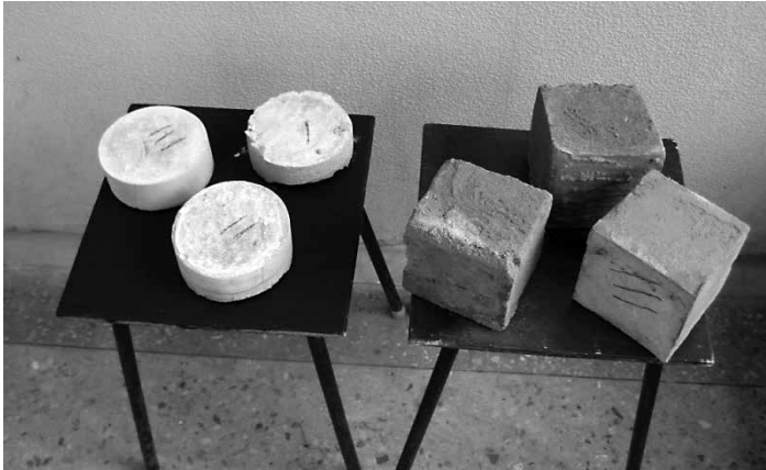
Figure 2.8. Solidified soil samples used for compressive strength and freeze thaw resistance studies
