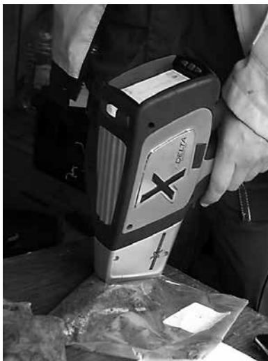
Figure 2.10. Portable DELTA Olympus Handheld XRF Analyzer in action (photo by F. Kaczala)
