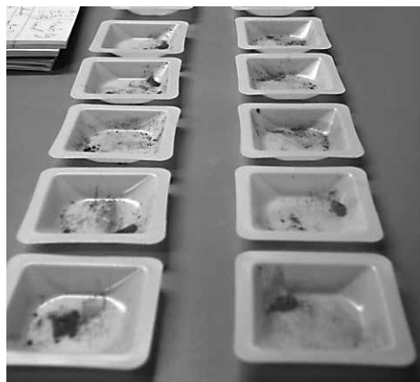
Figure 2.9. Modification of Devonian clay; modification with Na and Ca salts for sorption kinetics tests
