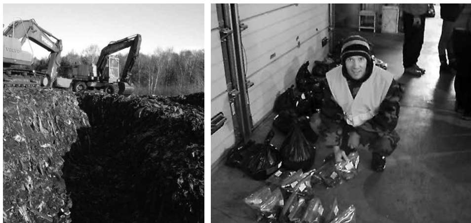
Figure 3.22. Sample extraction at the landfill – excavated, trommeled, shredded, sieved, manually sorted and fine fraction separated samples; derived for homogenization and analytical applications (from 16 tons to 16 grams) (author's photos)
