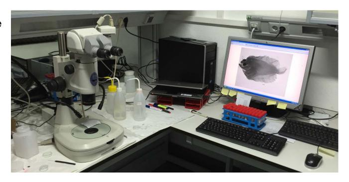
The **calibration factor** tells us how many pixels correspond to a millimetre for each microscope magnification
