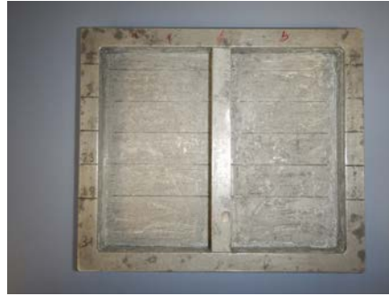
Figure 2.- Aluminum double mould used to embed otoliths.
