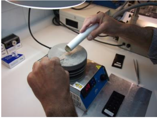
Figure 7.4.2.2.1 Sticking of the otoliths on the slide (left) and adjusting of the slide to the sanding piece (right).
