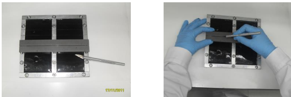
Figure 7.4.1.2.1.4. Marking of the cutting lines.
