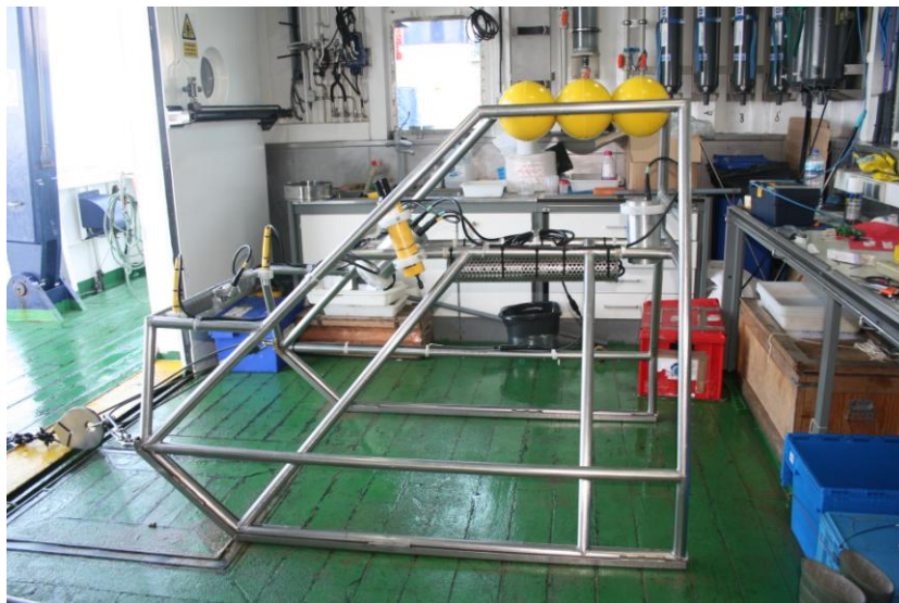
Figure 2. Sledge used during ISUNEPCA_0814 UWTW Survey in the Gulf of Cadiz ( Nephrops FU30).
