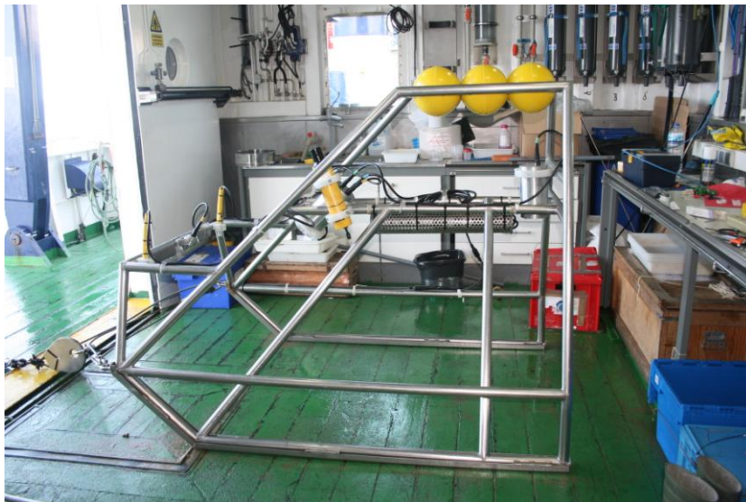
Figure 1. Sledge used during ISUNEPCA_0814 UWTV Survey in the Gulf of Cadiz ( Nephrops FU30).
