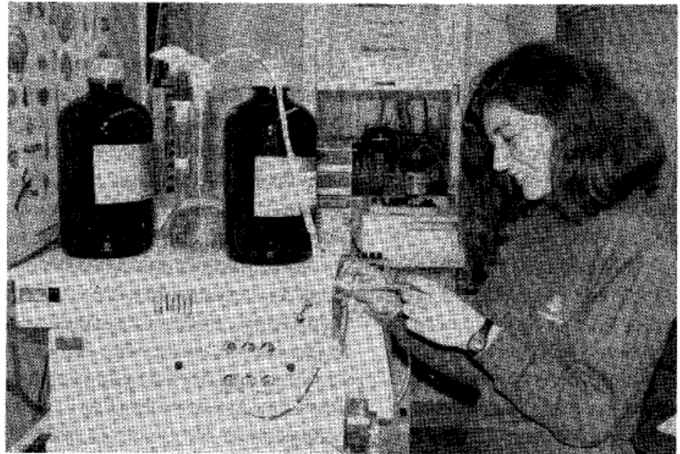
Nora Montoya (Argentina), a participant in the training course, injecting a sample in HPLC equipment for analysis of algal toxins.
