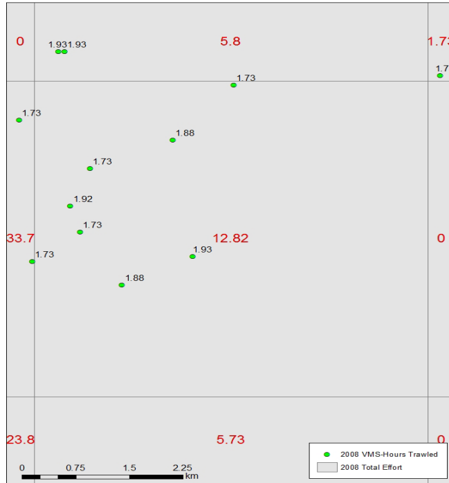
Figure 4.1.2.1.1: Sample calculation of total annual fishing effort. Green points represent filtered VMS pings and the hours related to each ping, and the red text is the total number of hours fished in the cell, based upon the VMS ping data.
