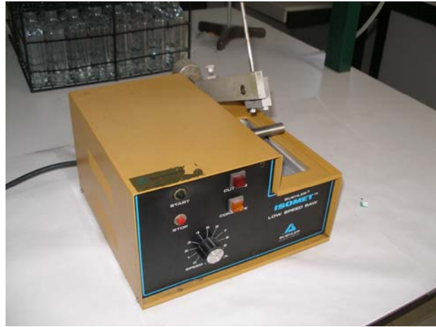
Figure 6. Diamond blade slow ISOMET saw cutter.
