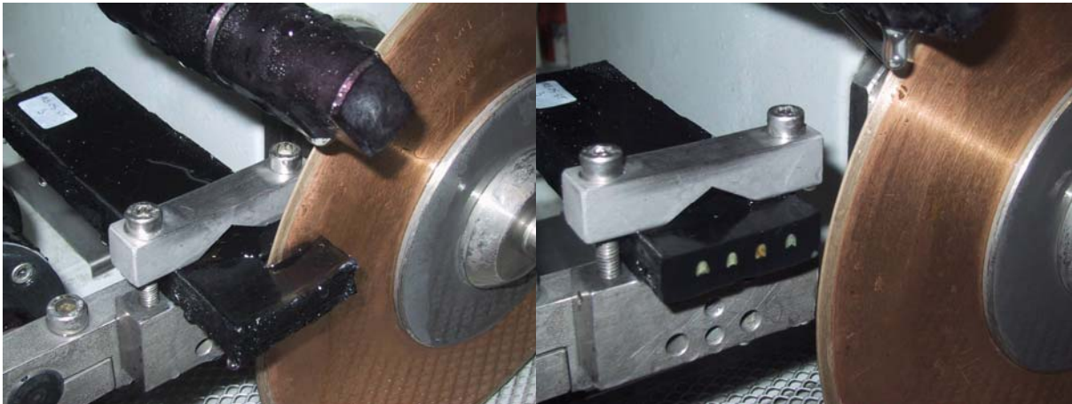
Figure 9 and Figure 10. Cutting a resin-moulded block of spines. ISOMED 5000 cutter. IEO ©
