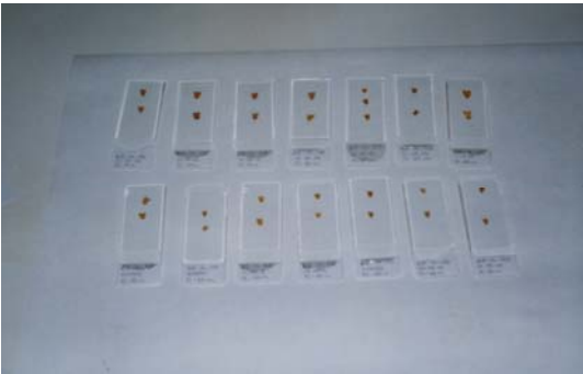
Figure 12. Sections on slide, embedded in epoxy resin. Air-drying.
