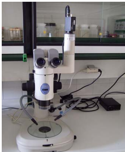
Figure 16. Binocular microscope with camera incorporated for image analysis.
