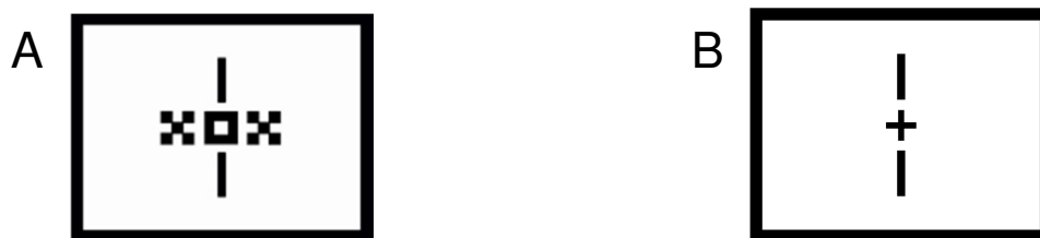
Figure 2.3. The fusion stimulus for fixation disparity (A) and vergence step response (B) measurement. The fusion stimulus (A: XOX; B: a central fixation cross and a peripheral frame) was presented to both eyes, either at baseline stimulus level (corresponding to the viewing distance) or at additional disparity (convergent or divergent).
