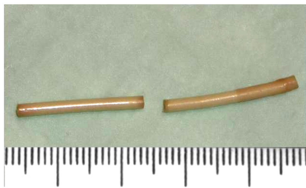
Fig. 2. Photography of broken implant removed.
