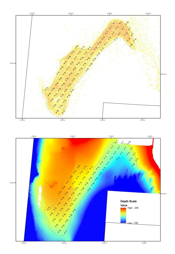
**Figure 1:** Porcupine Bank 2014 UWTV map of station positions overlaid on a heat map of *Nephrops* directed fishing (top panel) and bathymetry (bottom panel). The black polygon line indicated the ground boundary currently used.
