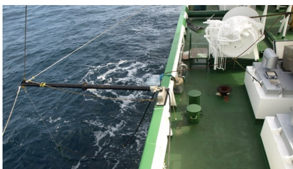
Figure 3. Towing boom c.3m long, with support stays.
