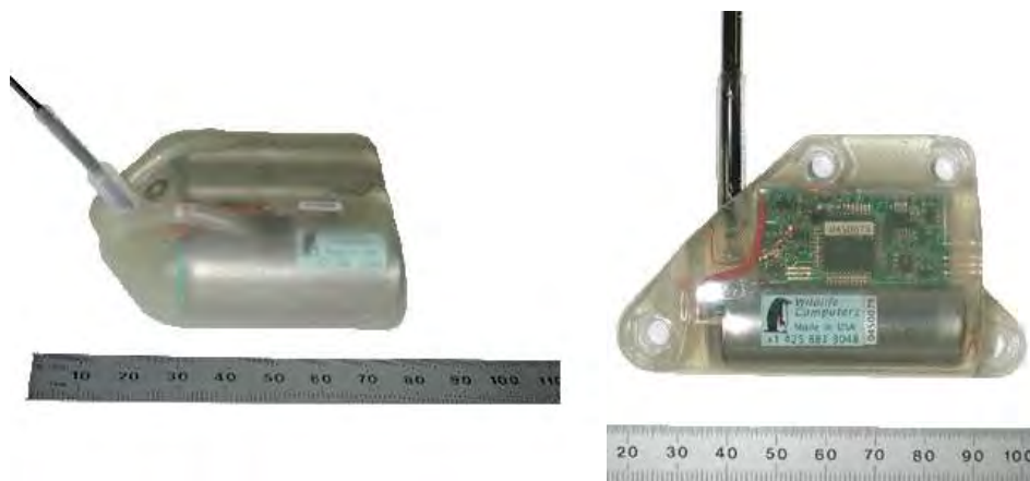
Examples of marine GPS tags and SPOT tags from Wildlife Computers
