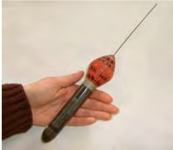
PAT Archival tag from Wildlife Computers, used on basking sharks
